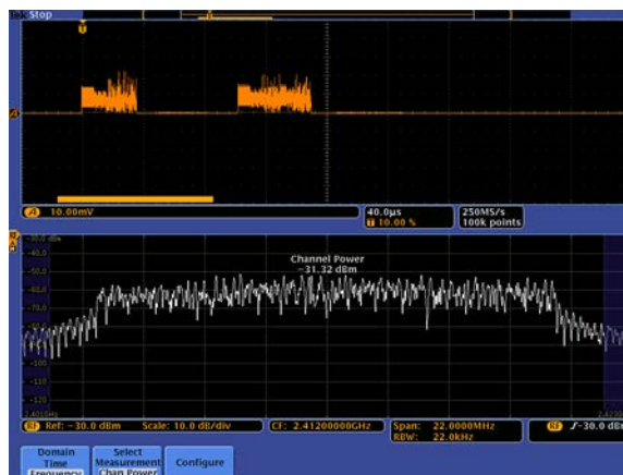
Automated channel power measurement of first burst in Wi-Fi transmission
